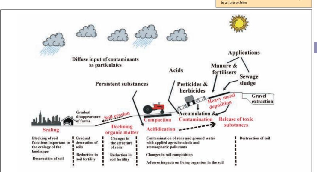
The process and inter-relationships of soil degradation. Decline in organic matter may cause erosion, facilitate compaction, decrease water infiltration and increase the danger of floods and landslides (RJ).
