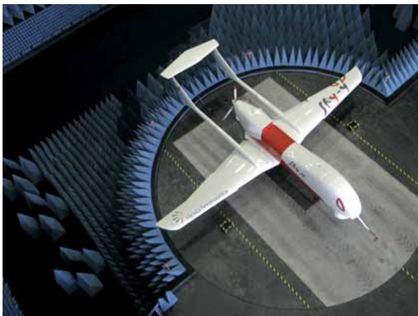
Alenia Aeronautica's Sky-y (UAV) ready for EMC testing inside Anechoic Chamber
