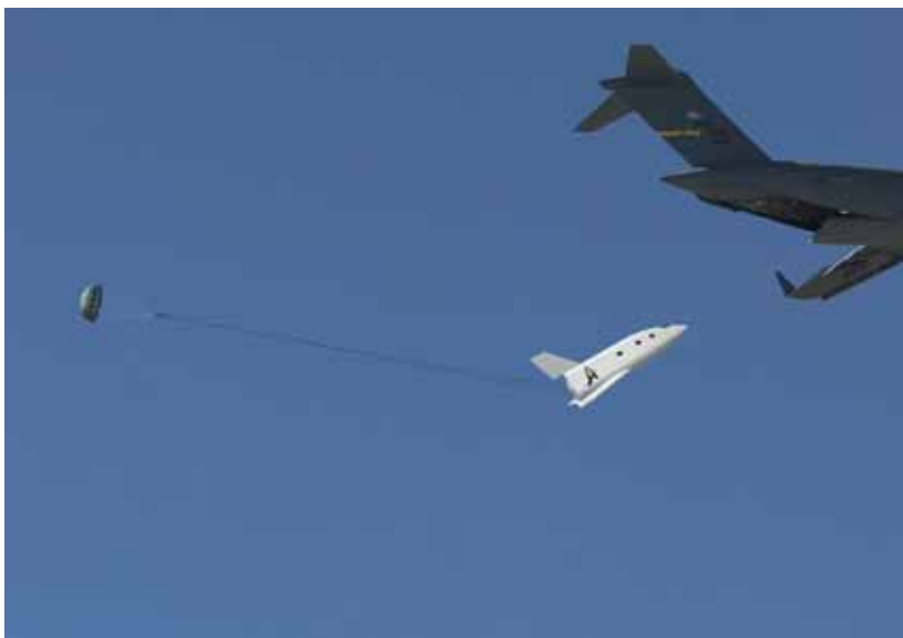
ALPHA, hybrid propelled vehicle launched at high altitude for short-range flights (here: one of several launch options).
