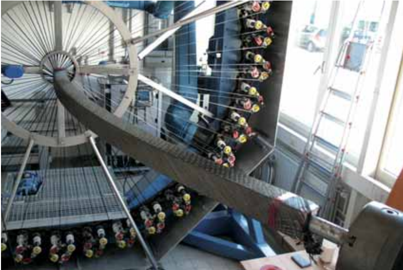
Manufacturing of the Carbon Fibre Preform for a Curved Profile by Braiding
