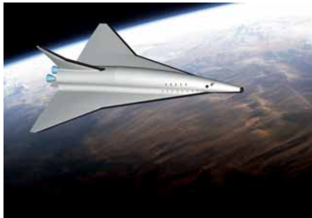
SpaceLiner, two-stage all rocket propelled vehicle launched vertically from ground for ultra-fast long-range flights.
