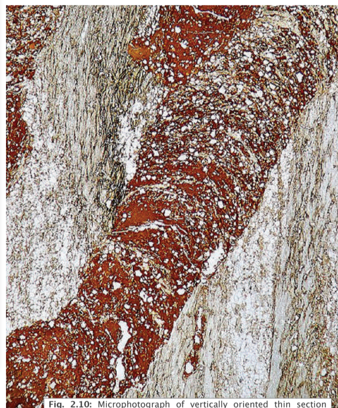
Fig. 2.10: Microphotograph of vertically oriented thin section showing a channel and chamber formed by soil fauna. (EAF)
