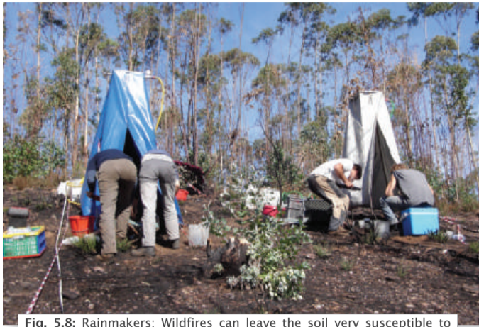
Fig. 5.8: Rainmakers: Wildfires can leave the soil very susceptible to both water and wind erosion processes, one of the main components of land degradation and desertification. Here, scientists are simulating rainfall, after a wildfire in a Eucalyptus plantation, and measuring soil erosion by water. (MM)
